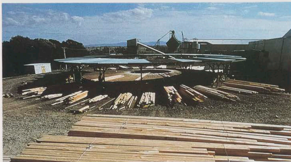
Left: The circular sorting table at Fletcher Timber's Kopu sawmill where timber is selected and stacked according to size and grade. The mill now cuts timber to Japanese specifications.
