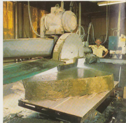
Mr Malcolm Moore operates a 48-inch diamond saw to shape a slab of Hinuera stone.
