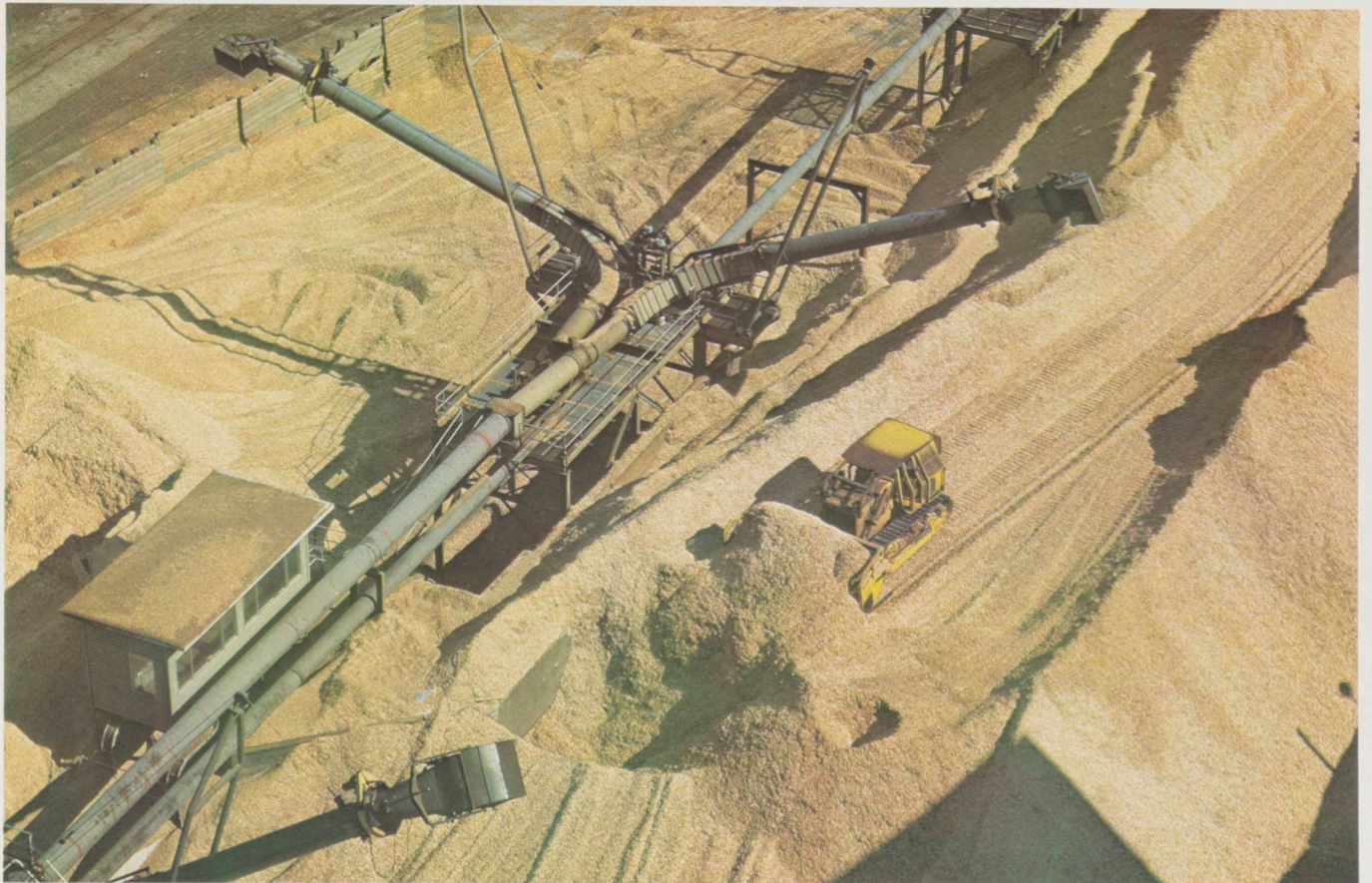
The wood chip storage area. From here the chips to be processed into long-fibred chemical pulp for export are fed by conveyor to the continuous digester.
