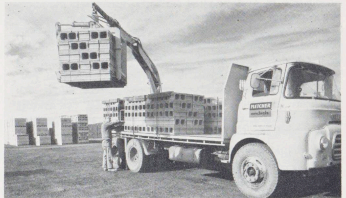
Above: Sales Director, R. A. L. McLean, in discussion with Production Director, K. R. Simmonds. Below: Boom gear for loading and unloading ensures mechanical handling right to the site.
